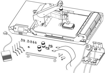
Rework Station with 110W IR under heater (80x60mm²) and automated SMD placement process by Auto Vision Placer (AVP), incl. Easy Solder software package and DBL 06 control unit with six high resolution sensor inputs for thermocouples (Type K).
