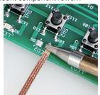
Solder removal for through-hole components
