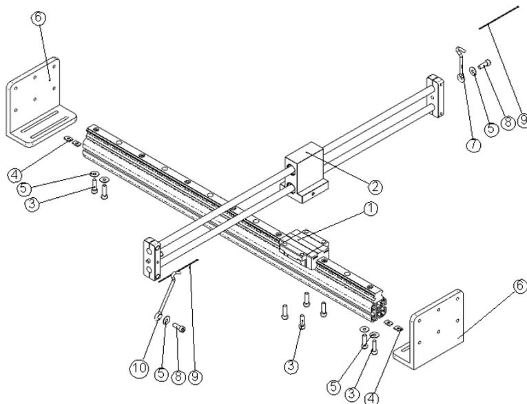
Mount the In-line stand according to the below picture. Adjust height of the stand for 240 mm working distance (Distance between PCB and front edge of HD camera).
